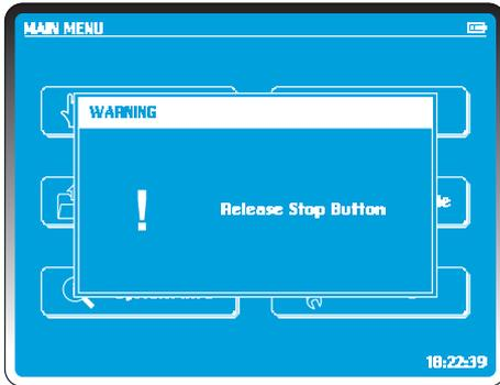
The Red Emergency **Stop / Pause** button can be pressed at any time. A stop signal is broadcast and all current and future operation of modules is paused.
