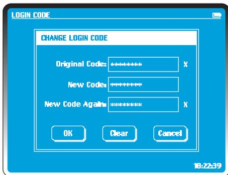
Using the keypad enter the code and select **OK**. If you make an error an 'X' is displayed on the right side of the code box. Use the **Clear** button to delete entries.
